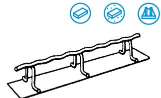
Dayton Superior's Beam Bolster is used to support lower beam steel from the soffit form. Legs are spaced on 2-1/2" centers. Available in 1-1/2" to 5" heights in 5' lengths. Manufactured in bright basic, plastic protected, galvanized, epoxy coated or stainless steel protected.
